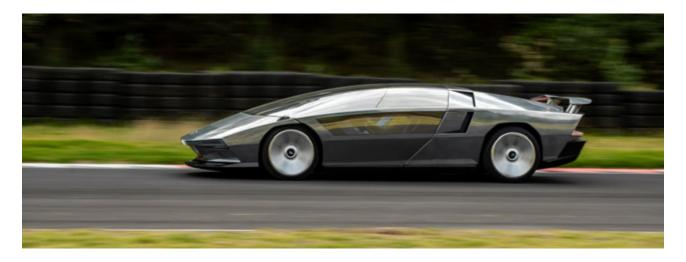
The only nonaluminum parts are the front spoiler, rear diffuser and side sills, all of which are made of exposed carbon fiber. The rear is characterized by the integrated spoiler that lifts up and the taillights that are hidden underneath: when lit they create an interesting "shadow light" effect.
