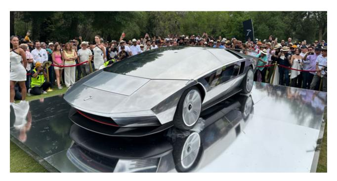
The Peralta S, a mid-engine, rear-wheel-drive sports car, is a futuristic car made entirely by hand from fully exposed, mirror-polished aluminum, with the special feature that there is no visual difference between the glazed surfaces and the body, creating a monolithic effect.
